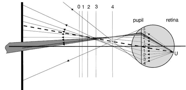
Fig. 6. The shaded region represents the bundle of rays that enter the sight-hole aperture. In this figure we have modeled a myopic eye with positive spherical aberration. The rays from point U on the retina cause illumination of the region from 2.5 to 3.1 mm on the pupil. The illumination distribution across the pupil is calculated for each point across the retinal point spread, and the distributions are summed together to yield the retinoscopic reflex for a single source position.
