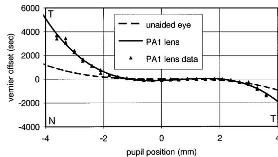
Fig. 10. Transverse ray aberration data for subject AR's left eye with and without the PA1 varifocal contact lens measured with the modified Ivanoff apparatus.<sup>30</sup> The unaided eye (dashed curve) has a nearly symmetrical aberration along the horizontal meridian. The PA1 lens induces a higher degree of aberration, particularly on the nasal edge. The symbols represent the actual data for the measurement of the transverse aberration. N, Nasal; T, temporal.
