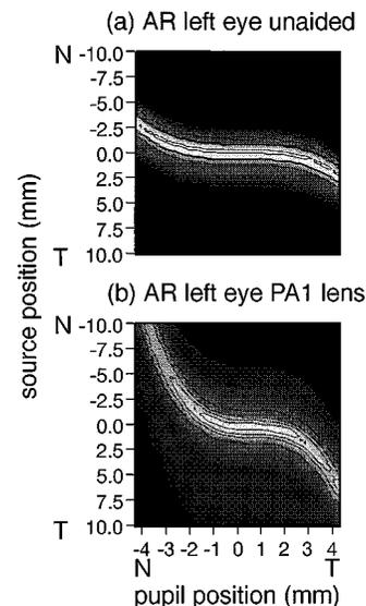
Fig. 11. Retinoscopic prediction for subject AR with and without the PA1 contact lens. The contour plots demonstrate that the retinoscopic predictions are measurements of the transverse ray aberration. Both contour plots are the retinoscopic predictions for the eye paraxially focused on the sight-hole aperture. N, Nasal; T, temporal.
