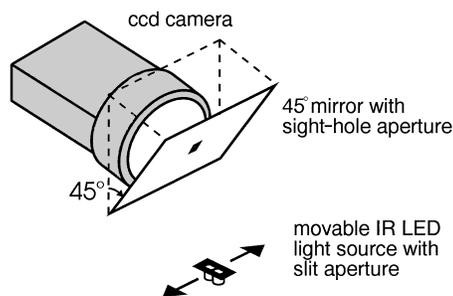
Fig. 8. Apparatus for CCD streak retinoscopy. The light source is composed of two adjacent infrared LED's set behind a slit aperture. The mirror is fully reflecting, except for a transparent sight hole 1.5 mm wide in the center. A micrometer stage is used to vary the source position with respect to the sight hole. The CCD focuses through the sight hole onto the pupil of the subject.
