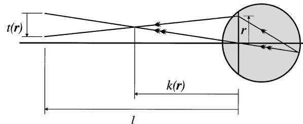
Fig. 3. A ray (single arrow) emerging from a retinal point passing through the exit pupil at a radius  $\mathbf{r}$  crosses the principal ray (double arrows) from the same point a distance  $k(\mathbf{r})$ . The transverse aberration,  $t(\mathbf{r})$ , is a measure of the emerging ray intercept position from the principal ray intercept in a plane perpendicular to the optical axis at a specified distance  $l$  from the exit pupil.
