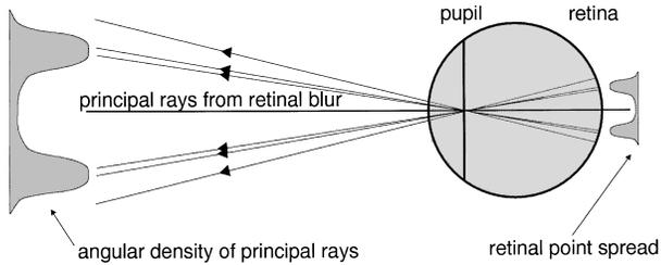
Fig. 5. Principal rays emerging from the blur on the retina. In the first step of the analysis we determine the principal ray emerging from each point on the retinal blur. This construction shows that the angular density of principal rays is a scaled equivalent of the blur on the retina (from Roorda *et al.*<sup>22</sup>).
