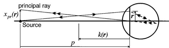
Fig. 4. Determining the principal ray. The dashed rays inside the eye are not necessary for determining the position of the principal ray and are used only to clarify the illustration. The principal ray is drawn from the center of the exit pupil and intersects the incoming ray at the specific far point  $k(\mathbf{r})$  for the radius  $\mathbf{r}$  at which the ray enters the eye.
