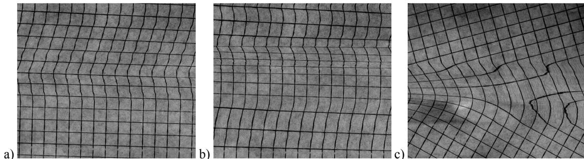
Figure 1: Illustration of the distortions produced in scanned images by a) horizontal, b) vertical, and c) torsional rotations of the target during a single scan.
