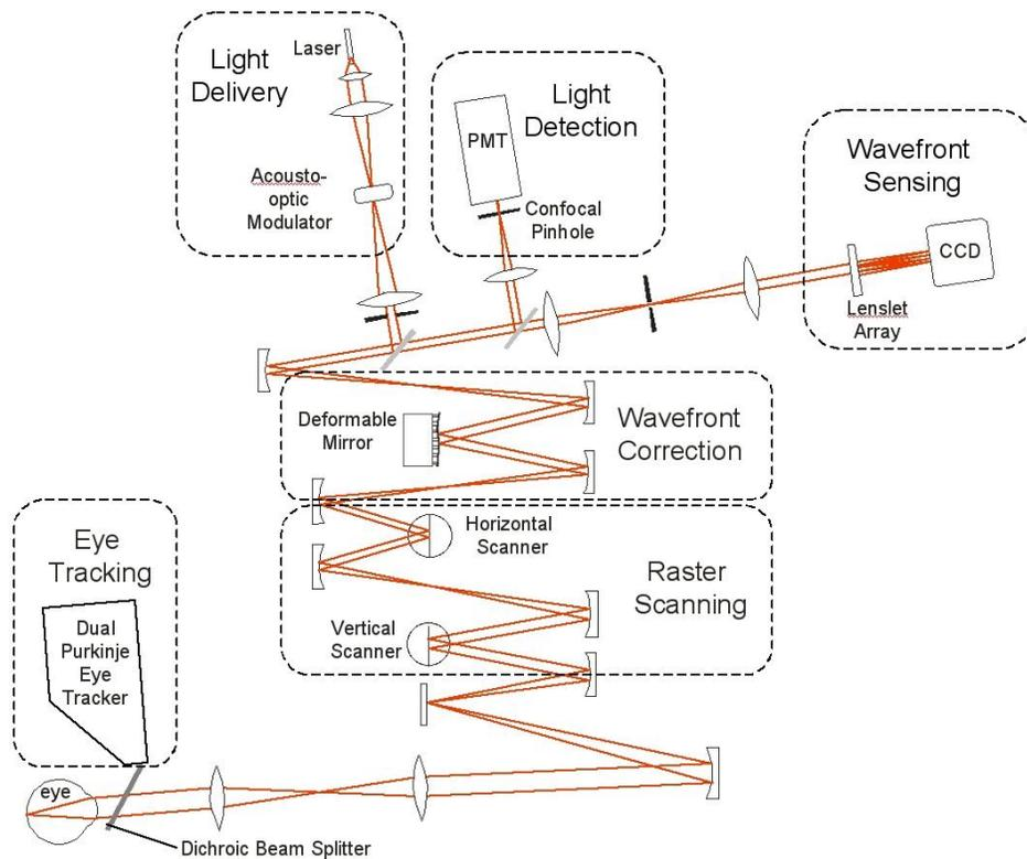
Figure 3. Schematic of the Adaptive Optics Scanning Laser Ophthalmoscope, modified with an additional relay telescope to accommodate the dual-Purkinje image eye tracker. The dPi tracker uses infrared light to track rotations of the eye on horizontal and vertical axes. The dichroic beam splitter passes visible light and reflects infrared, allowing both systems to operate without interference. PMT photomultiplier tube.
