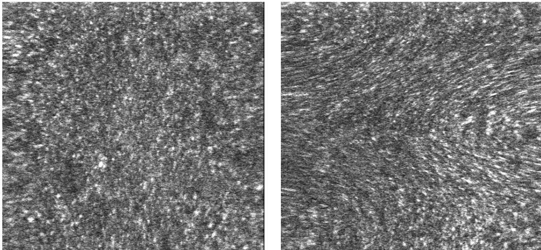
Figure 2. Successive frames from an AOSLO video recording of the foveal region of a human retina. The field size was one degree square. The image on the left is typical of most frames collected, with relatively little distortion due to eye movement. The frame on the right has a pronounced shear distortion due to a rapid horizontal rotation of the eye.
